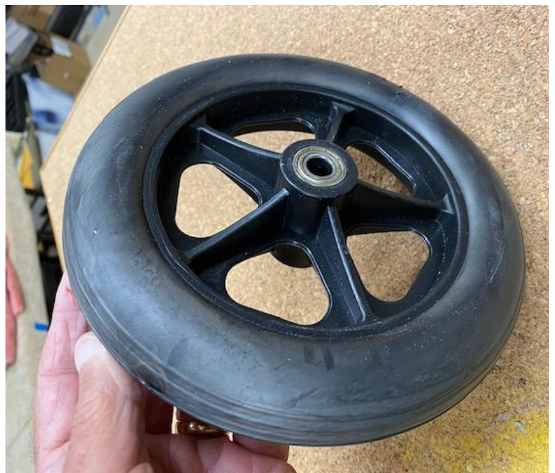
Here's the modified wheel after the tread was removed. This photo also shows the Delrin bushing. The tread was removed by mounting the wheel on my drill press and turning it using 60, 80 and 120 grit sand paper. I found that a light touch with the sand-paper, using no block, avoided any out of round problems.
