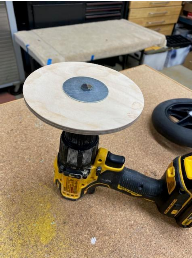
The picture on the left shows the tool used to make the slightly domed wheel covers. A disk of quarter inch plywood with a bolt was chucked in a hand drill held in my vice. Then a ring of sixteenth ply was glued to a circular piece of quarter inch balsa and turned to the proper shape with sand paper.
