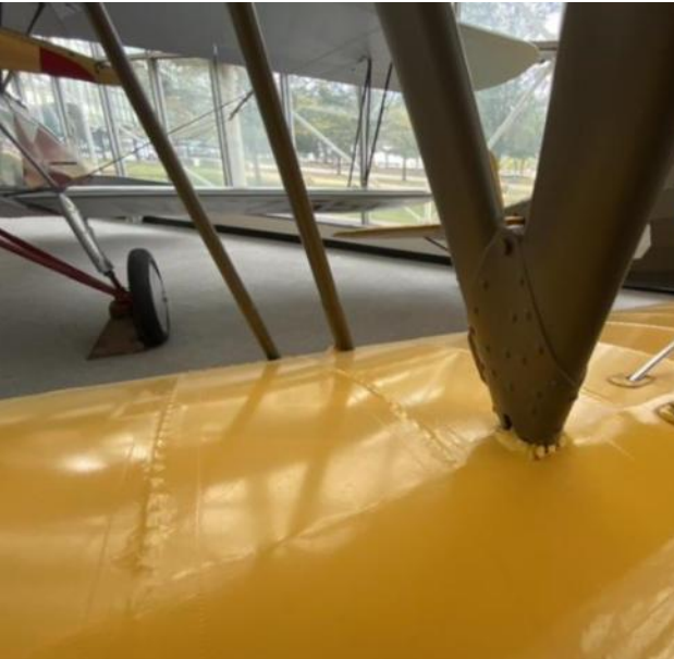
Here's the full scale rib stitch detail. These planes had very close stitch spaces of only one inch since they were pretty fast aircraft. And here's a shot of my upper wing stitching and tape detail.
