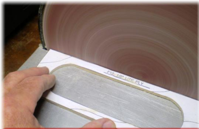
Finish the cut by sanding away half of the line with a disk sander.
