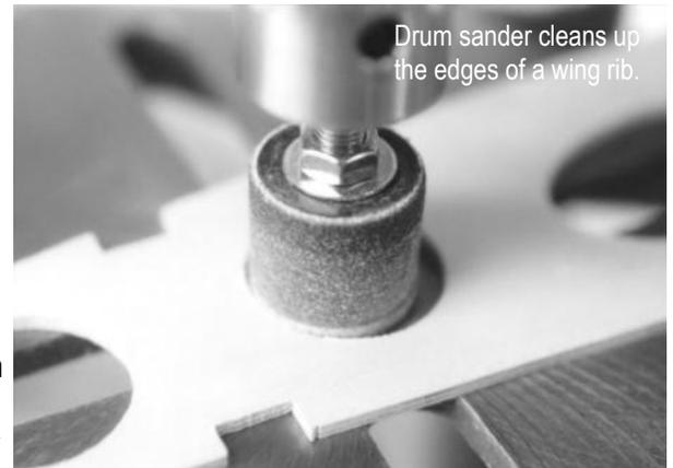
Drum sander cleans up the edges of a wing rib.
